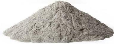
Rosswag Engineering is the first TÜV SÜD certified manufacturer of metal powders for additive manufacturing. Thanks to a complete in-house process chain including powder atomization, a complete AM material qualification can be carried out within a few weeks.
