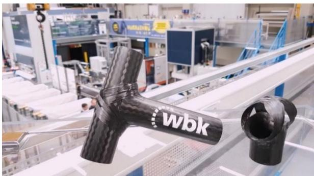
Thanks to a continuous virtual process chain (CAE chain), the flexible **joining process** involving filament winding offers new possibilities for the production of lightweight hollow profiles. The idea is based on bamboo joining techniques which have been used successfully in Asia for centuries. The bamboo poles are joined by crossing and winding ropes around the nodal points of the poles (cf. illustration).
