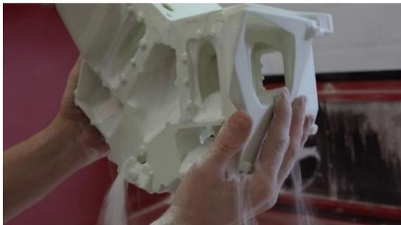
The 3D printed master model made of plastic maps out the contour of the future metal component inside the ceramic casting mold.
