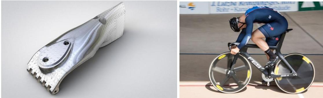
Captions: (left) The SLM procedures is well suited for the production of metal components with complex geometries. / (right) After the development and testing stages, the handlebar stems could be completed and delivered to the athletes within two months. Sources: 3D-Laserdruck Photos in a higher resolution and other motives are available from [mirko.hertrich@leichtbau-bw.de](mailto:mirko.hertrich@leichtbau-bw.de) or can be downloaded from <http://www.leichtbaubw.de/en/press/releases.html>.
