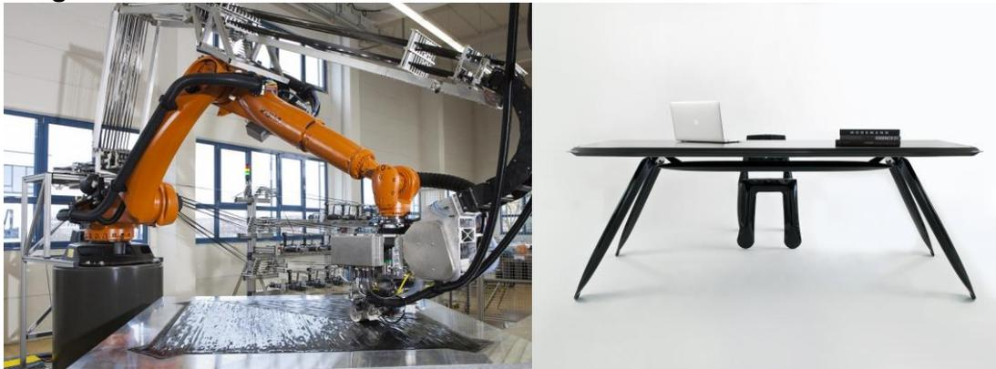
Caption: **(Left)** Compositence GmbH's RoboMAG-T machine places load-path optimised thermoplastic tapes on a form with minimum cutting scrap. / **(Right)** The fiber-fair placement process with the RoboMAG system can create very interesting surface appearances. One example is the carbon table top Nogi, which Compositence produces itself with process designer Oskar Zieta. Pictures: Compositence GmbH
