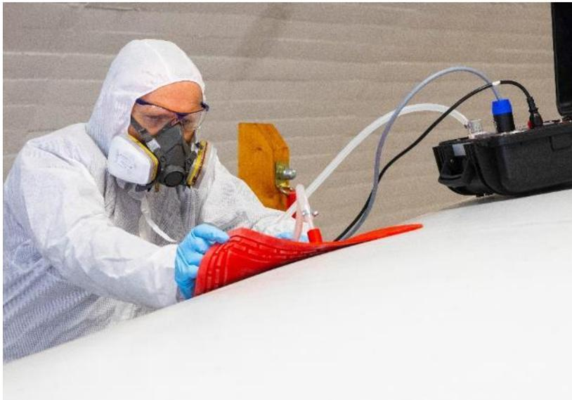
Repairing a fibre composite structure: The mobile repair unit is visible at the top right, and the heating blanket is placed straight on top.
