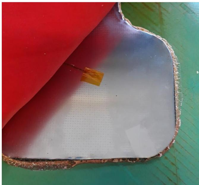
Clearly visible: The sheet is cut to size as a susceptor to deliver targeted heat to the damaged area.
